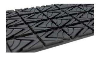
Rubber pulley lagging refers to the layer of rubber that is bonded to the shell of a conveyor pulley. Its purpose is to protect the shell of the pulley from damage, increase friction with the conveyor belt and dispense water off the pulley.
