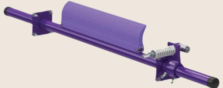
*Belt cleaners are an important aspect of your conveyor belt system because of their ability to reduce carryback – the material that sticks to the belt after it leaves the discharge of the head pulley and builds up underneath the belt. The will protect and maintain your system.*
