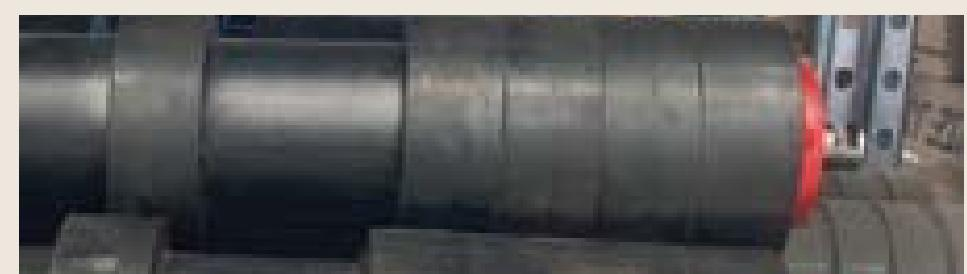
**HDPE.** Poly idlers and return rollers (with options of HDPE, PVC or nylon shells) are used for corrosive environments, or the belts are carrying a sticky product.
